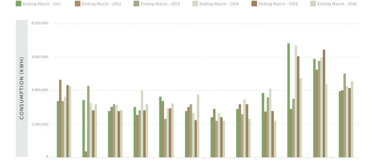
Manager, helps the Javits Center monitor consumption. The above chart shows year over year monthly comparisons for kWh consumption. From this information, it can be determined in which months the most electricity is used, and if, over time, that consumption has decreased. Overall consumption metrics are run against different variables such as gross square footage days, heating degree days and cooling degrees
